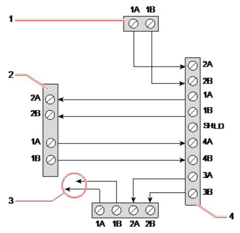
Wiring of a branch expander
