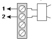
Internal sounder wiring (12V)
