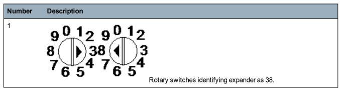
For a system with automatic addressing, expanders and keypads belong to the same numbering sequence. For example, expanders and keypads are automatically numbered 01, 02, 03, etc., by the controller in the order in which they are detected, for example, its relevant location to controller. In this configuration, zones are allocated to each input expander.
