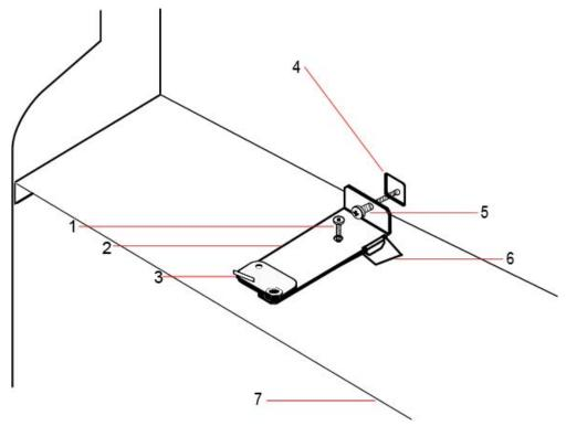
6. Install the lid on the housing to test the tamper switch connection. Lift the lid by approximately 1mm to activate the tamper switch.
