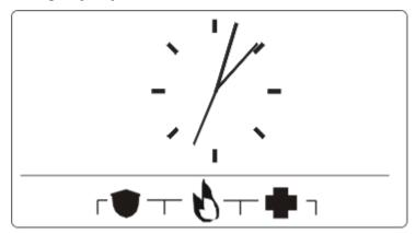
Depending on configuration, emergency keys are displayed. A simultaneous pressing of the keys activates an emergency call.
