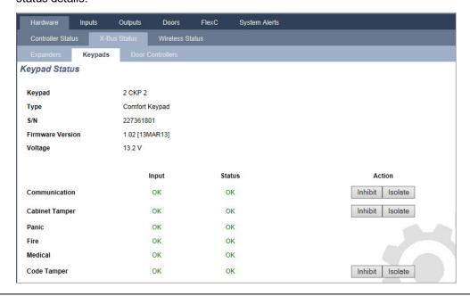
Communication The physical status (OK, Fault) and the programmed status (OK, Isolated, Inhibited) of the keypad cable connection to the expander.
