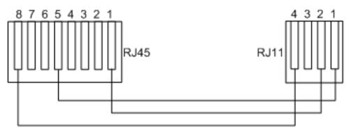
X10 wiring to the controller
