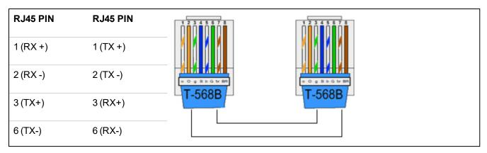
Use the crossover cable for connecting the SPC controller directly to a PC.
