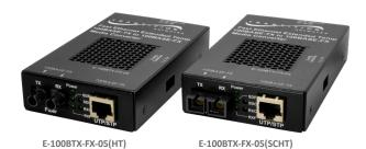
The E-100BTX-FX-05(HT) is a Hardened Ethernet stand-alone media converter that provides an interface between 100Base-TX ports and 100Base-FX ports, allowing users to integrate fiber optic cabling into extreme 100Base-TX copper environments, by supporting an operating temperature range of -25°C to 65°C. Operating at Layer 1, the physical layer, data is passed through the converter at line speed, making it ideal for applications where low latency is essential.
