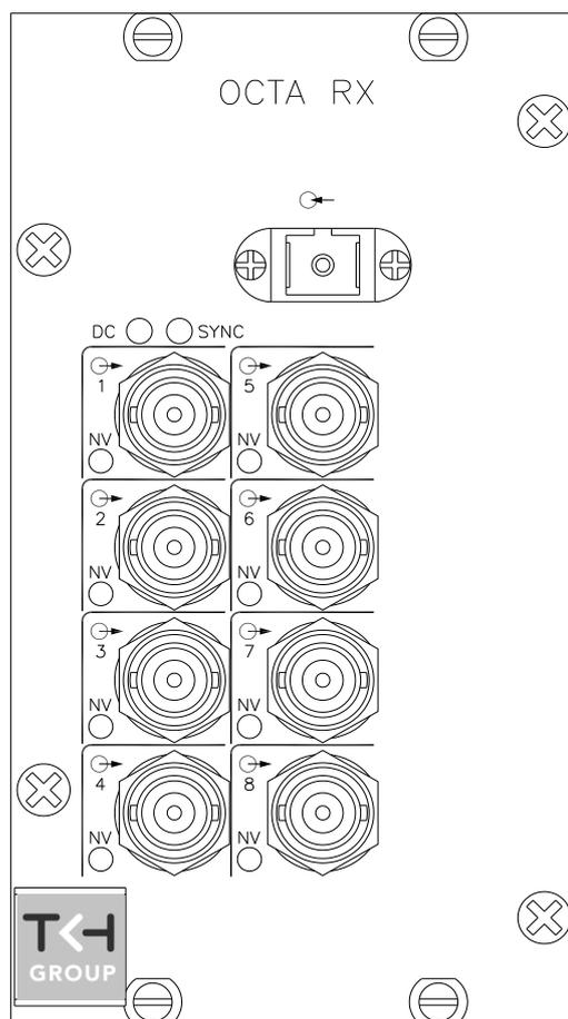
Figure 1. OCTA 40x0 RX front panel. TX panels look similar, with video inputs instead of outputs. See Table 1.
