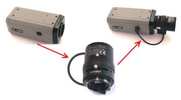
Mount a lens onto the BC840
