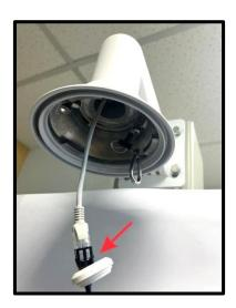
**NOTE**: Please thread the Ethernet cable straight through the grommet. Do not bend the Ethernet cable as it may cause damage to the grommet.
