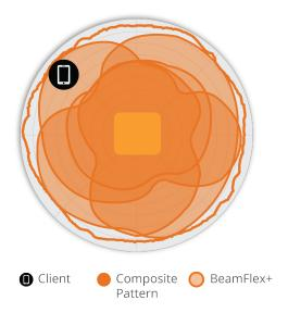
Figure 2. R610 2.4GHz Azimuth Antenna Patterns
