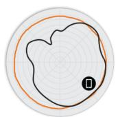
Figure 3. R610 5GHz Azimuth Antenna Patterns
