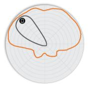
Figure 5. R610 5GHz Elevation Antenna Patterns
