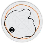
Figure 4. R610 2.4GHz Elevation Antenna Patterns
