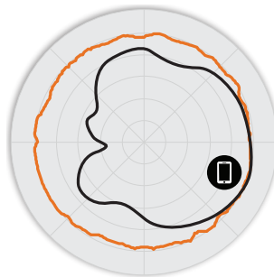
Figure 3. R510 5GHz Azimuth Antenna Patterns
