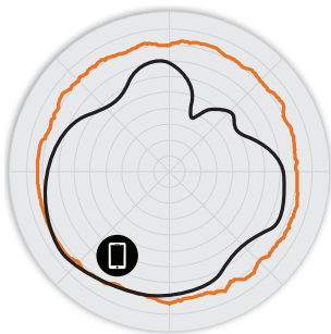
Figure 2. R510 2.4GHz Azimuth Antenna Patterns
