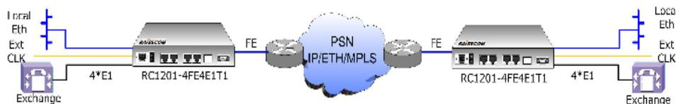
Point-to-point E1 and LAN extension over Packet Switching Network
