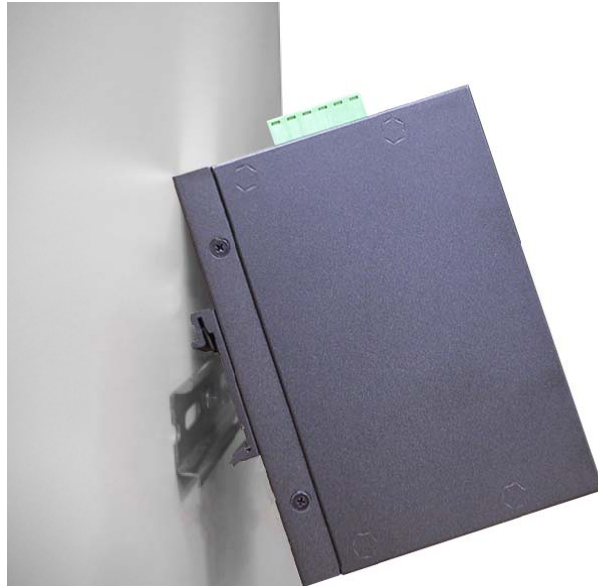
Fig. 4: Installation to DIN-Rail Step 1
