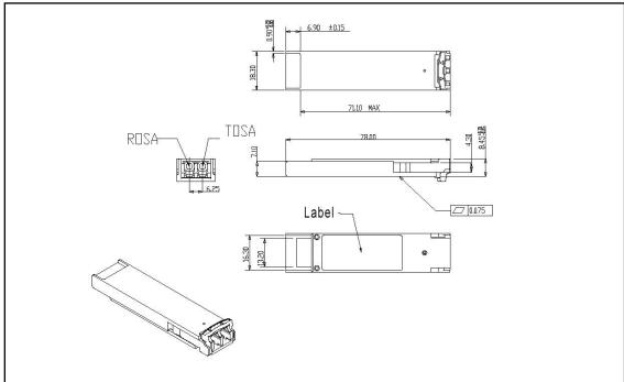
Figure3. Mechanical Specifications
