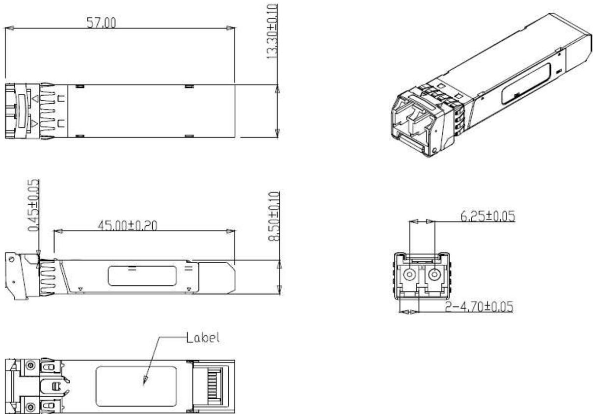
**Figure5. Mechanical Specifications**
